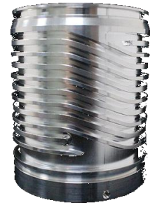
Five axis machining spiral groove
